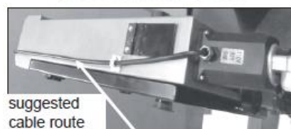
suggested cable route - Tracé du câble recommandé
